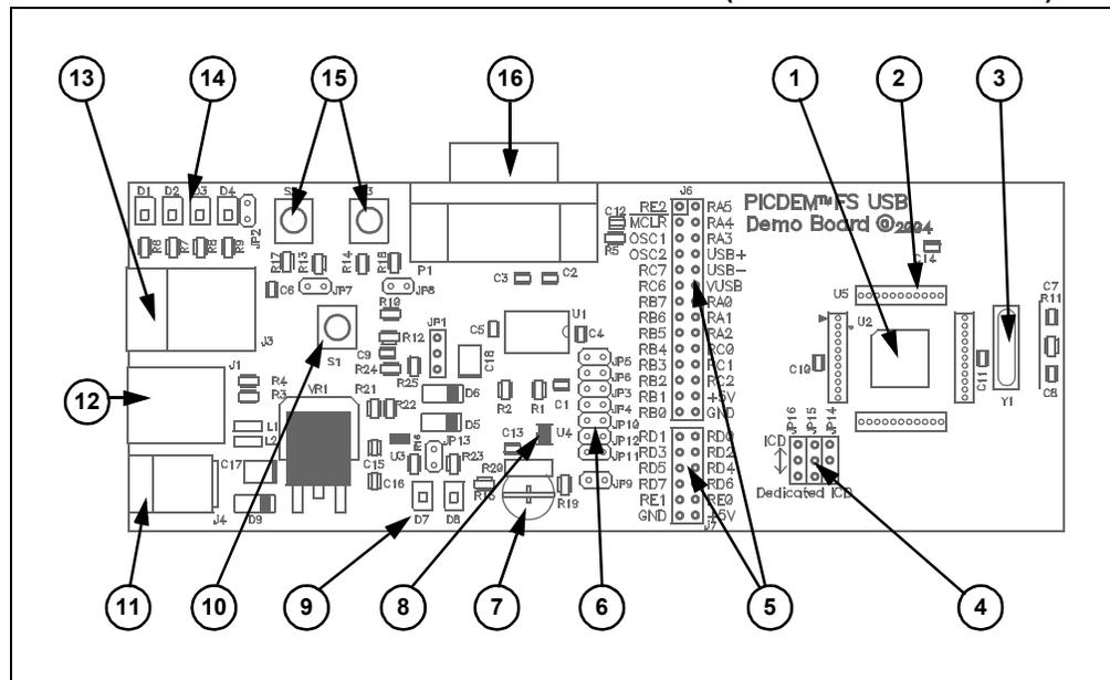
1. **Microcontroller:** The 44-pin TQFP PIC18F4550 microcontroller (U2) is the heart of the demonstration board, and provides all USB functionality on one chip. Refer to the device data sheet (DS39632) for a complete discussion of the microcontroller and its feature set.
