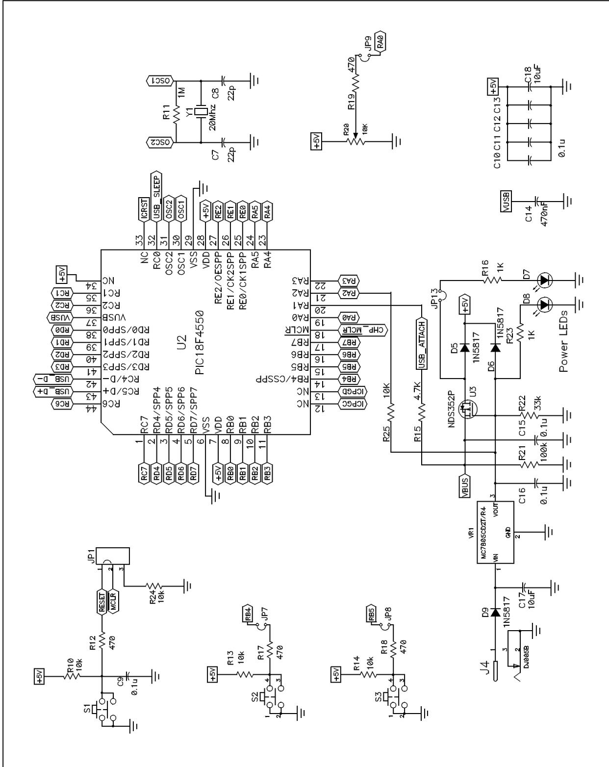
**FIGURE A-3: BOARD SCHEMATIC, PART 2 (USART, USB INTERFACE, THERMAL SENSOR AND STATUS LEDs)**
